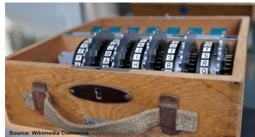
Figure 7. Extra rotor box for up to seven wheels.
