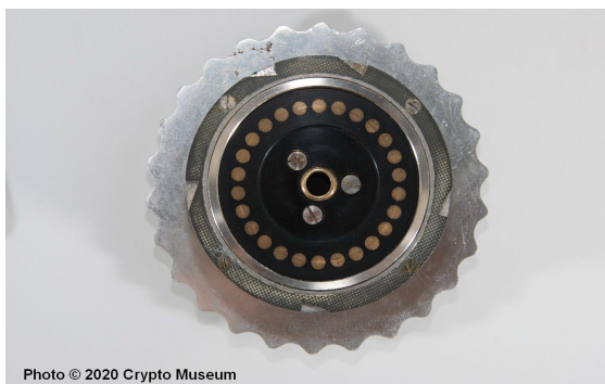
Figure 10. Enigma T wheel with five notches.
