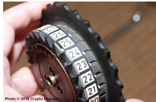
Figure 11. Variable notch rotor.
