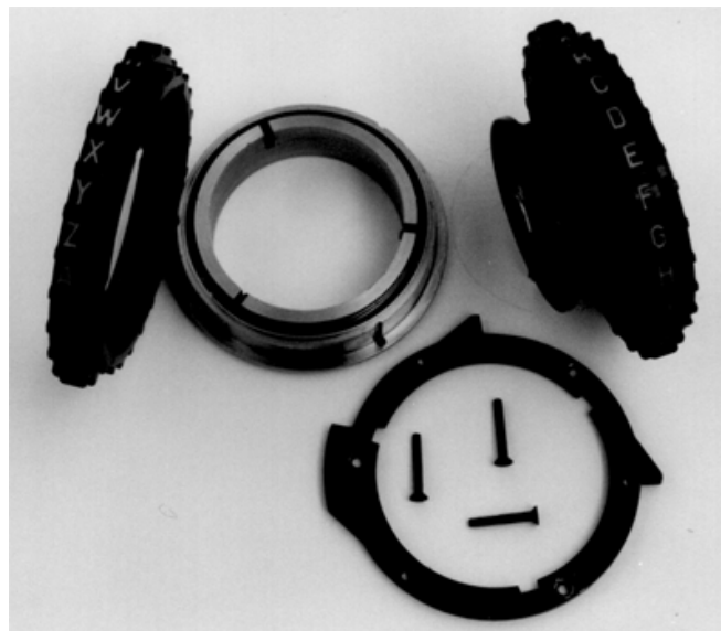
Figure 5. A contact wheel and drive wheel assembly shown disassembled into its component parts. From left to right: drive wheel letter ring, drive wheel body, notch ring (No. 12) with fixing screws and wired contact wheel assembly.
